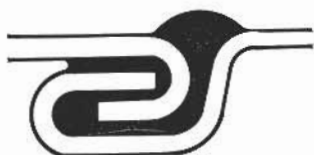
Figure 10. — Joint agrafé et brasé tendre
